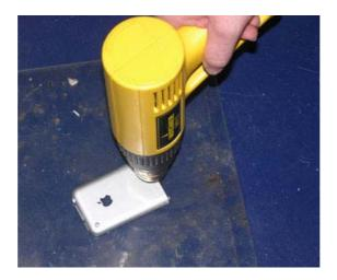
Generally the metal Apple logo will be the first to drop off, followed by the screw bushing at the base, then the outer parts of the frame.
