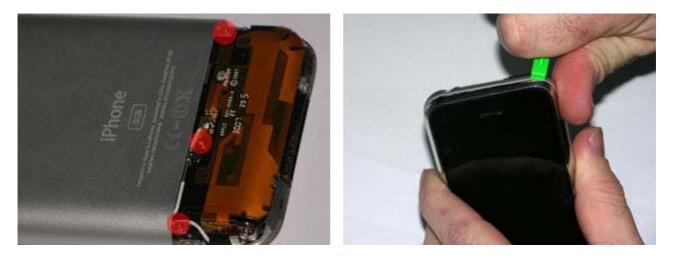
As with the antenna cover, start by running the opening tool along the edge of the phone, between the case and the chrome bezel until they start to separate, then gradually increase the gap between the case and bezel until the case comes off.
