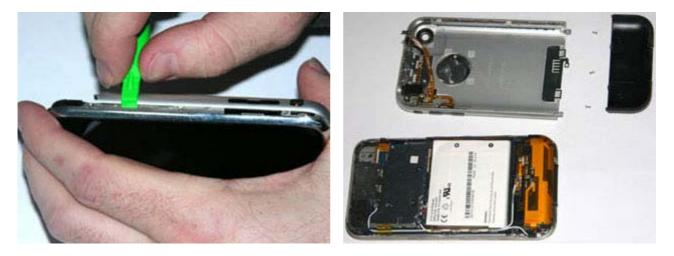
Try not to damage any inner parts of the metal casing as you will need these later. Once you are done, you should have something looking like the picture on the bottom right.
