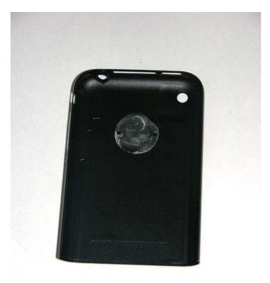
We used superglue gel, as this gives you a small bit of extra time to position the parts before they are bonded, also by using superglue, you will be able to clean off any excess glue with nail varnish remover.
