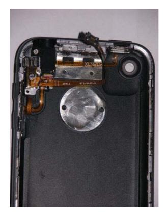
Reconnect the headphone circuit to the phone before putting the case back on in order to test the buttons by powering the phone on, then switching the silent button and adjusting the volume, making sure that each switch works correctly.
