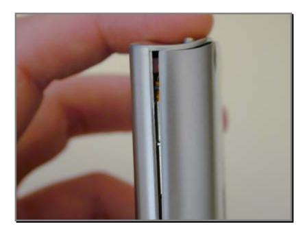
Run your finger nail all the way along the seam to the bottom of the case.
