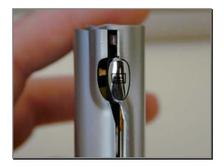
This should now allow the back of the case to be totally removed, the battery connector will easily disconnect, as it is just snap clipped onto the main board.
