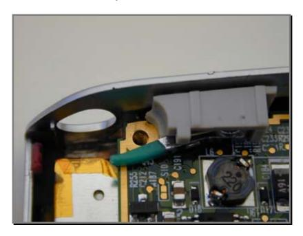
Next peel the Kapton tape from the backing paper and attach it onto the iPAQ main board, as show in the picture below, this insulates the metal stylus latch from the iPAQ main board.
