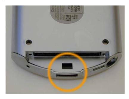
Gently clip the two halves of the casing back together, they should click easily back together. Then reinsert and tighten the four main case screws. Remember to slide the power switch back to the on position if you turned the unit off.
