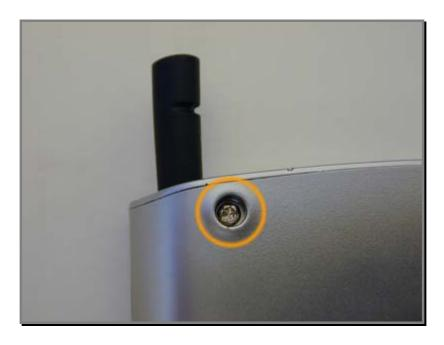
Proceed using a Torx size 6 screw driver to undo all four main case screws. If you do not have a Torx screwdriver available, a small jewellers cross head screwdriver can also be used.
