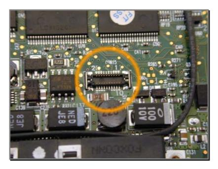
Once the battery connector firmly is attached to the main board you are now ready to re-attach the iPAQ's back casing.
