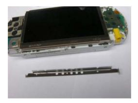
Do not take the lower button circuit off its metal mounting frame, although not a fatal error, this causes difficulties when reassembling the PSP as you have to re-align the circuit with the buttons.
