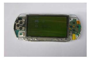
Make sure you remove the plastic film on the screen absolutely last before reattaching the front case, as this will prevent any dust getting onto the screen, which can be quite distracting whilst playing games.
