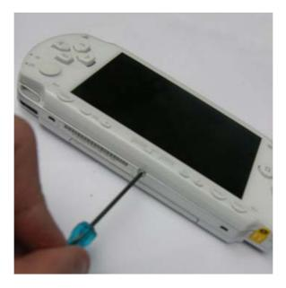
Slip on the front case and put all the screws in their original places, replace the battery and your screen replacement is complete.
