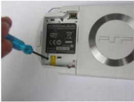
Finally, remove the screw at the base of the console next to the barcode sticker. The front case will just lift off allowing you to access the inside of the PSP.
