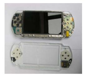
The Screen is protected by the lower button circuit which has to be removed in order to access the screen below. Start by un-hooking the circuit from the connector on the action button circuit board, this is a delicate operation as the latch is fragile and can snap easily.
