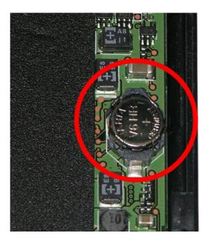
Use a small tool such as a jewellers flathead screwdriver or a credit card corner to pop out the backup battery from its holder on the logic board.
