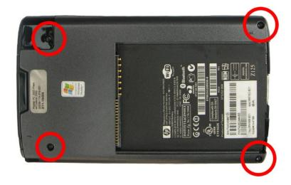
The rear case should just unclip allowing you access to the units logic board.
