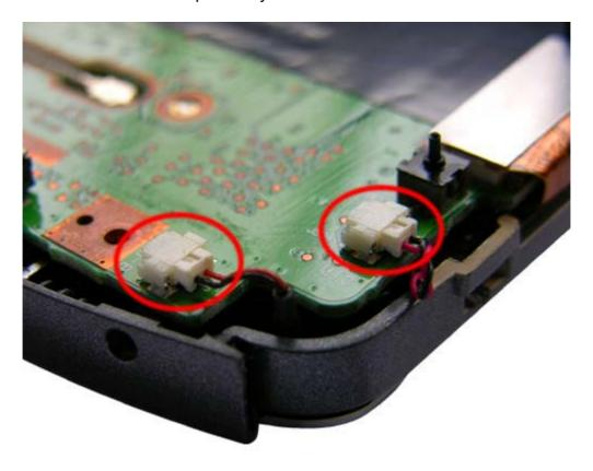
Disconnect the cable connectors on the left hand side of the unit also.
