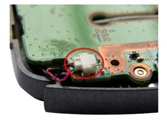
Disconnect the Screen cable by simply pulling the connector away from the socket.
