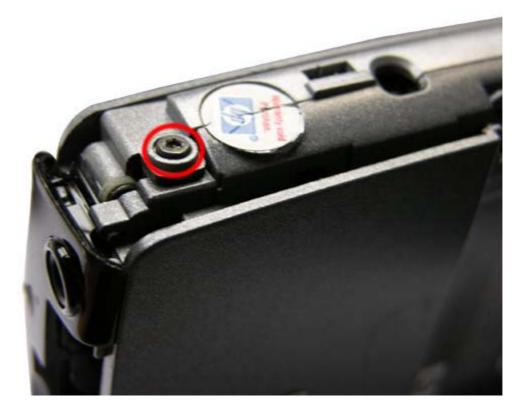
The case is now ready to come off, simply pull the front case away from the back case from the bottom of the unit.
