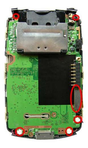
The first step is to disconnect the cable connectors on the right hand side of the unit, these cables simply pull away from the socket.
