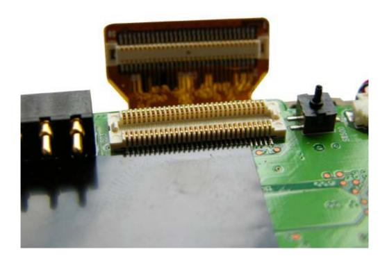
With these components disconnected you only need to unscrew the top two screws, after this the mainboard is ready to take away from the unit.
