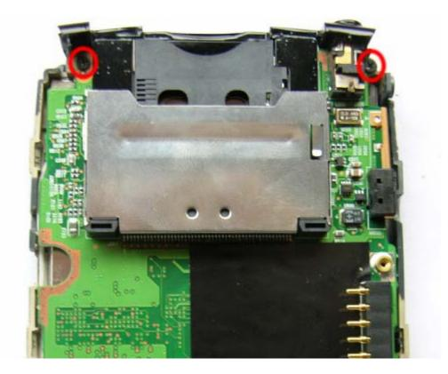
As the headphone socket (in the top left of the unit) also holds the unit into the case you will need to pull the mainboard downwards and away to release it from the front case. When removing the mainboard be aware that if your unit features the white WiFi cable you do not need to remove this in order to access the battery – it is long enough to allow you to replace the battery without disconnecting it.
