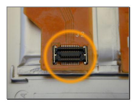
The battery connector shown above needs to be attached to the main board connector shown below the two just snap fit together.
