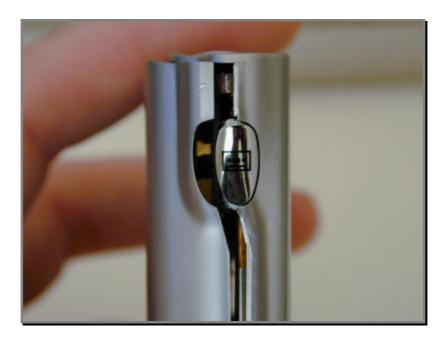
This should now allow the back of the case to be totally removed, the battery connector will easily disconnect, as it is just snap clipped onto the main board.
