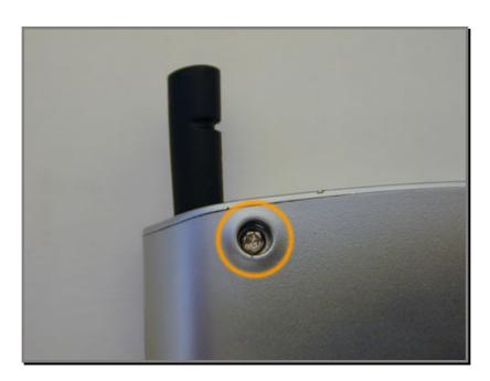
Proceed using a Torx size 6 screw driver to undo all four main case screws. If you do not have a Torx screwdriver available, a small jewellers cross head screwdriver can also be used. Remember to pop the stylus out as if you leave this in the silo it will prevent you from separating the case.
