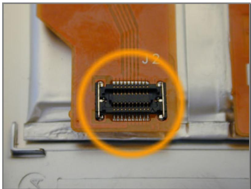
The battery connector shown above needs to be attached to the main board connector shown below the two just snap fit together.
