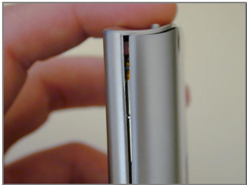
Run your finger nail all the way along the seam to the bottom of the case.
