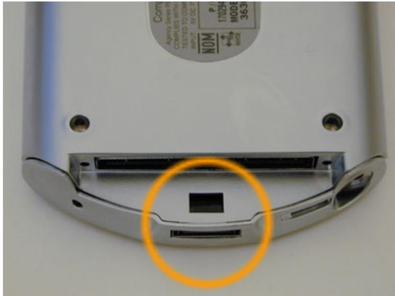
Gently clip the two halves of the casing back together, they should click easily back together. Then reinsert and tighten the four main case screws. Remember to slide the power switch back to the on position if you turned the unit off.
