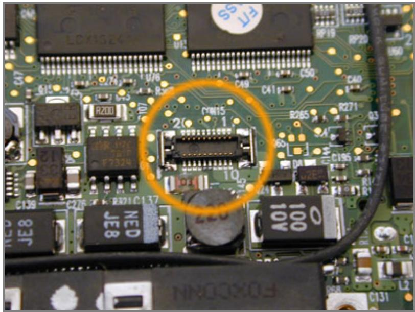
Once the battery connector firmly is attached to the main board you are now ready to re-attach the iPAQ's back casing.
