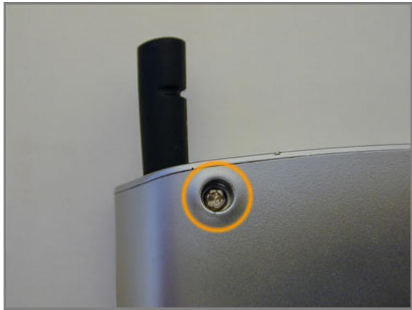
Proceed using a Torx size 6 screw driver to undo all four main case screws. If you do not have a Torx screwdriver available, a small jewellers cross head screwdriver can also be used. Remember to pop the stylus out as if you leave this in the silo it will prevent you from separating the case.
