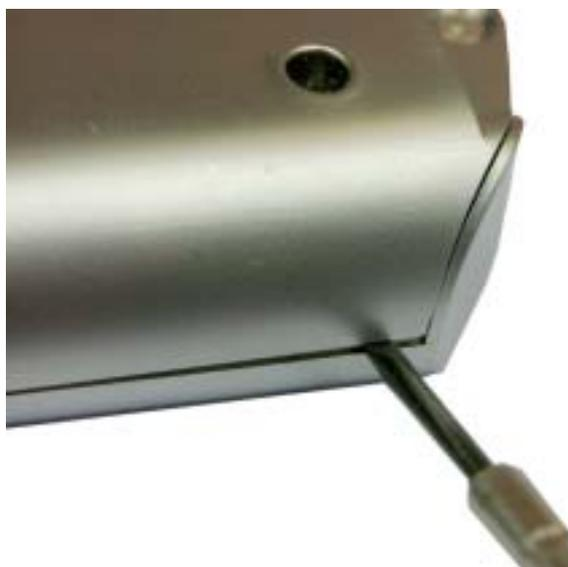
Once this corner is lifting, move your nail / screwdriver upwards to pop the rest of the case from the front.
