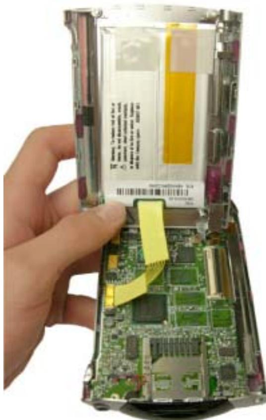
You will see that the battery rests in the rear case, which is in turn attached to the main board. You do not need to detach this yellow battery cable from the main board, simply disconnect it from the battery itself. This is done by carefully lifting it from the battery connector with your fingers.
